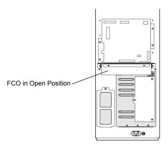
Figure 6-11 Fibre Channel Option in the Open Position
